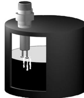
The heated RTD responds to the heat transfer coefficient of the media with which it is in contact. Gases with low heat transfer result in a high differential temperature between the heated and reference tips
