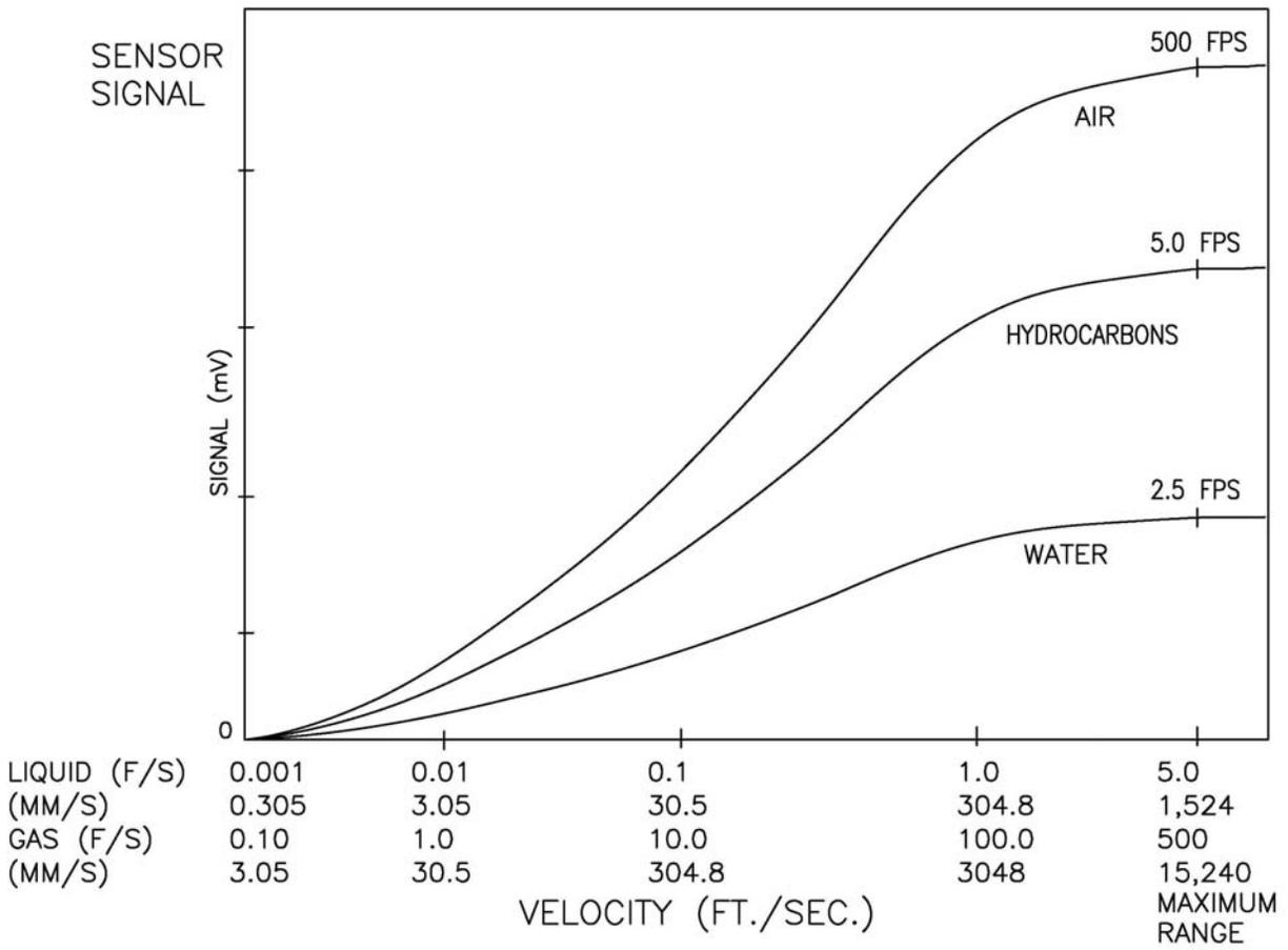
**FIGURE 2B microtuf® MODEL FS4200 FLOW RESPONSE FOR THREE MEDIA**
