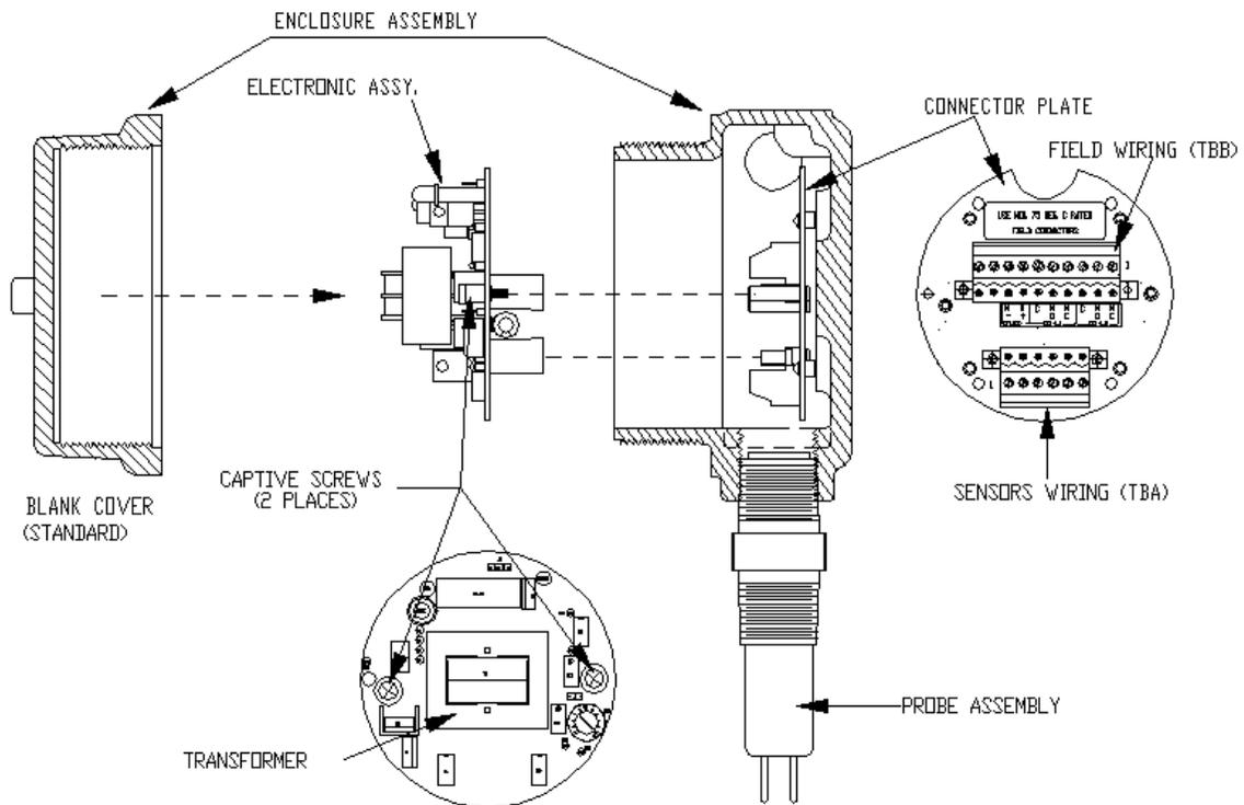
**FIGURE 4 microtuf<sup>®</sup> SWITCH ASSEMBLY (MTF400.DWG/.FCW)**
