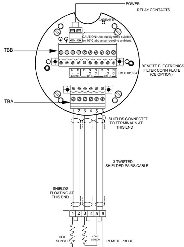
**FIGURE 6A microtuf<sup>®</sup> SWITCH REMOTE ELECTRONICS FIELD WIRING DIAGRAM (MTF6A00FCW/.DWG)**
