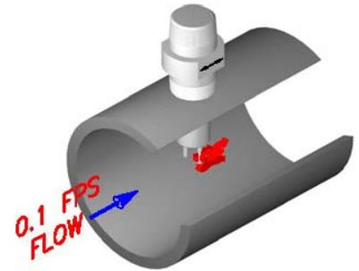
Flow across the tips decreases the thermal differential because of the higher heat transfer of flowing fluids. This differential is compared with the trip point.
