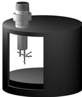
Note: Probe tips contain matched RTD's one of which is self-heated with about 400mw of power. The other provides temperature compensation
