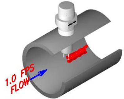
When flow is above the trip point the differential is smaller than at the set point and the relay and LED remain tripped.
