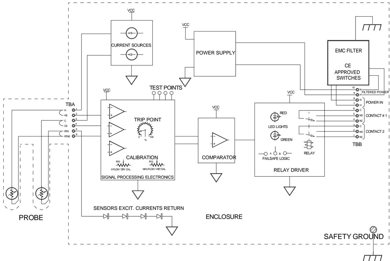
FIGURE 3B: MICROTUF MODELS WITH THE CE OPTION SWITCH BLOCK DIAGRAM (MTF3B00.DWG)
