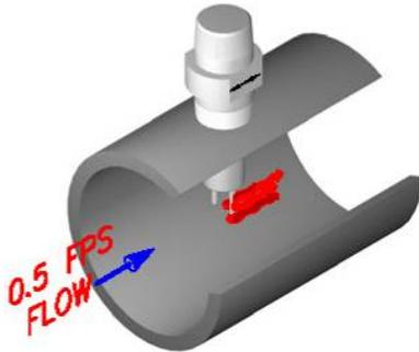
When the lower differential matches the customer select flow velocity trip point (set point) the switch relay and red LED are tripped.
