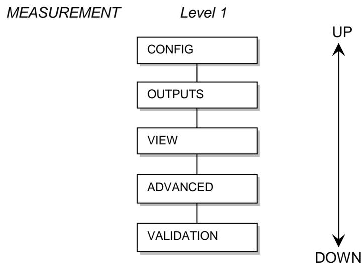
**Figure 3.1: Level One Programming Menu Structure**
