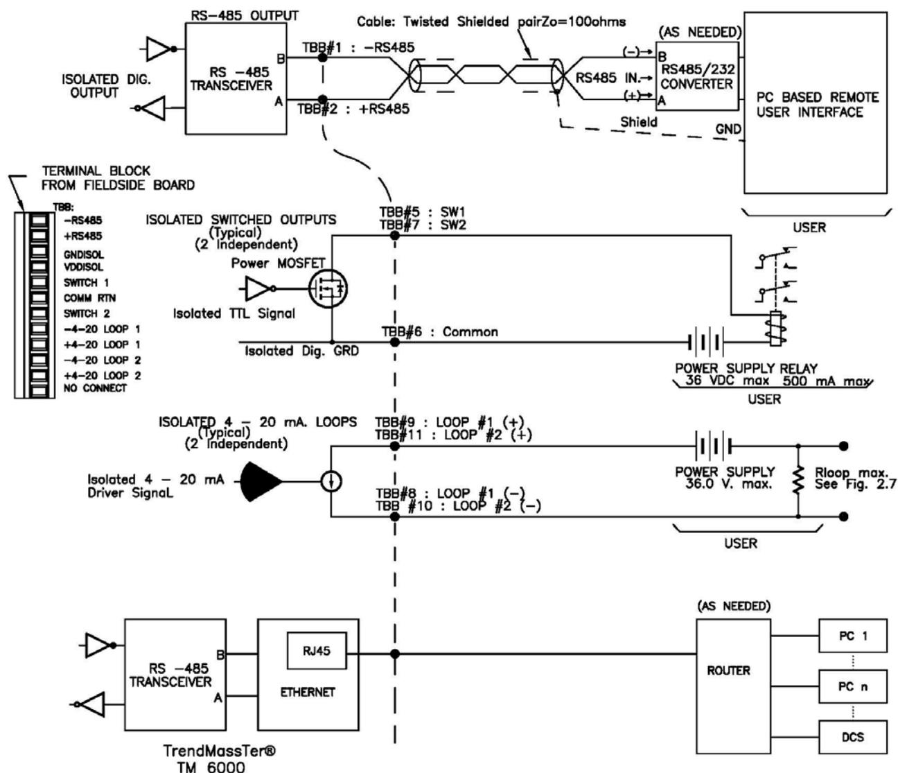
Figure 2.8: TrendMassTer® Outputs Wiring
