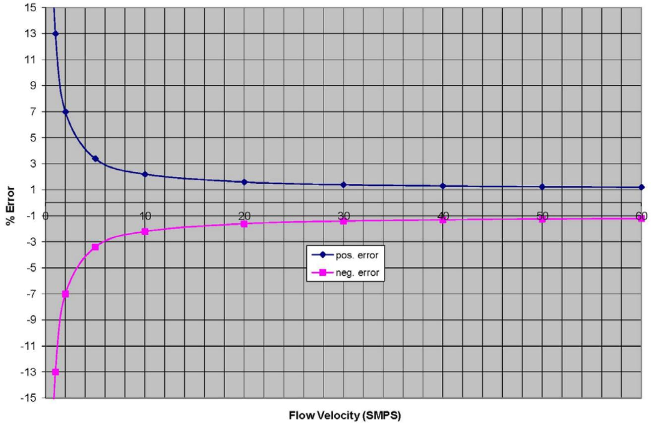
**Figure 5.1: Total Error Plot for the TrendMassTer® in Air
