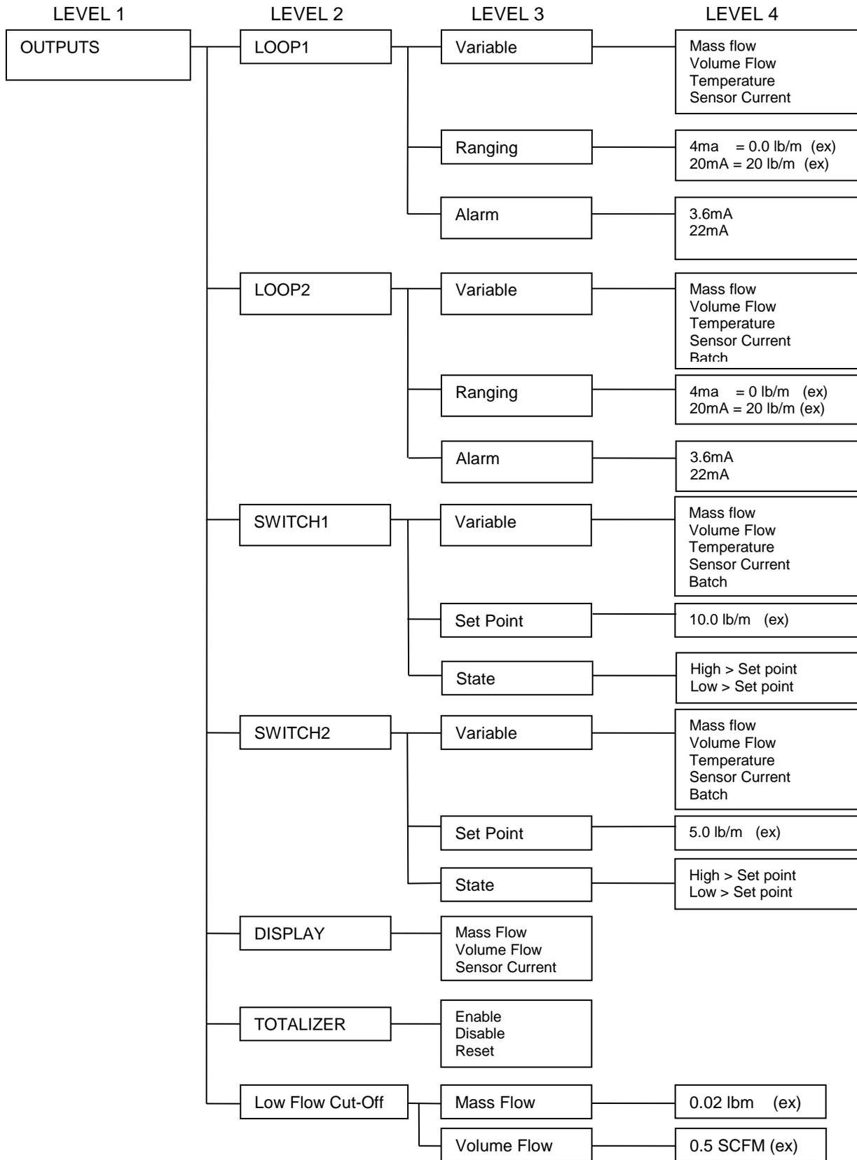
**Figure 3.3: OUTPUTS Menu Breakdown**
