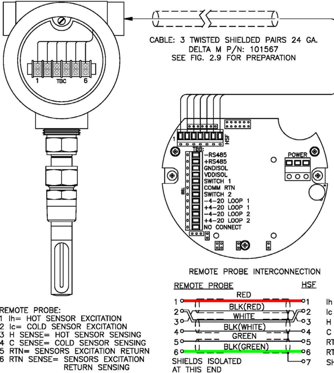
**Figure 2.5 TrendMassTer® Field Wiring For Remote Probe**
