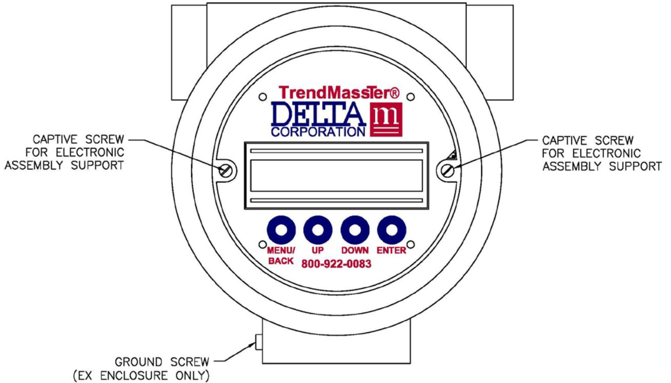
**Figure 2.2: TrendMasTer® Electronics Inside the Enclosure**
