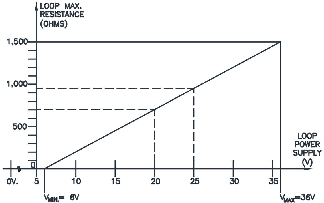
**Figure 2.10: Maximum Loop Resistance vs. Supply Voltage**
