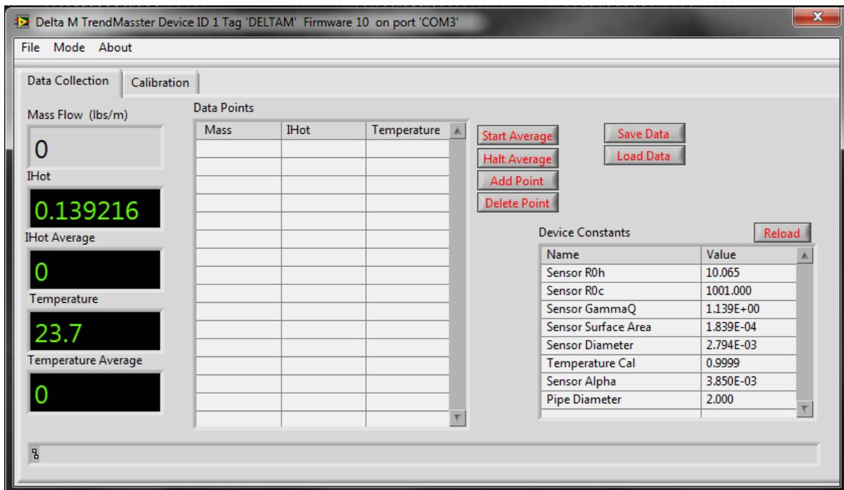
**Figure 3.10A: Calibrate Panel**
