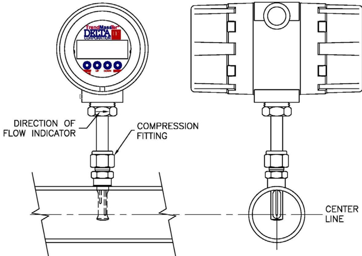
Figure 2.1: Probe Installation
